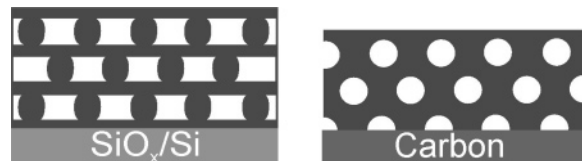
Figure 7. Sketches introducing symmetric wetting of the silicon substrate and the free surface by the PB (dark) component (left sketch) and asymmetric wetting conditions on the carbon coating (right sketch).
